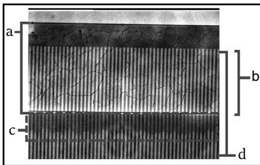
Figure 3, top: Image obtained from freezing experiment. (a) Microchannel containing bulk ice, identified by the grain boundaries present in image. (b) 500  $\mu\text{m}$  channel overlap. (c) Liquid water in nanochannels (darker region) coexisting with ice (brighter region) at subfreezing temperature. (d) Nanochannel array.
