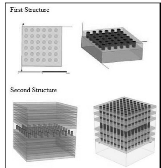
Figure 1: Schematic. Top, First Structure: The 1.5  $\mu\text{m}$   $\text{SiO}_2$  film was deposited, patterned and etched. The holes were 0.5  $\mu\text{m}$ , electroplated with Cu. Bottom, Second Structure: Alternative layers of  $\text{SiO}_2$  and Si are deposited, patterned and etched (all through the layers), then holes electroplated with Cu.
