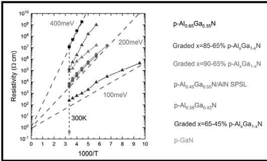
Figure 2, above: Temperature dependent TLM showed two orders less resistivity for graded AlGa<sub>x</sub>N structure over constant AlGa<sub>x</sub>N.
