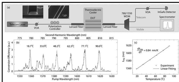
Figure 2: (a) Experimental setup. Insets are SEM pictures showing the waveguide facet and sidewall. (b) SHG spectrum at different temperature. (c) Measured  $\lambda_{PM}$  as a function of temperature.
