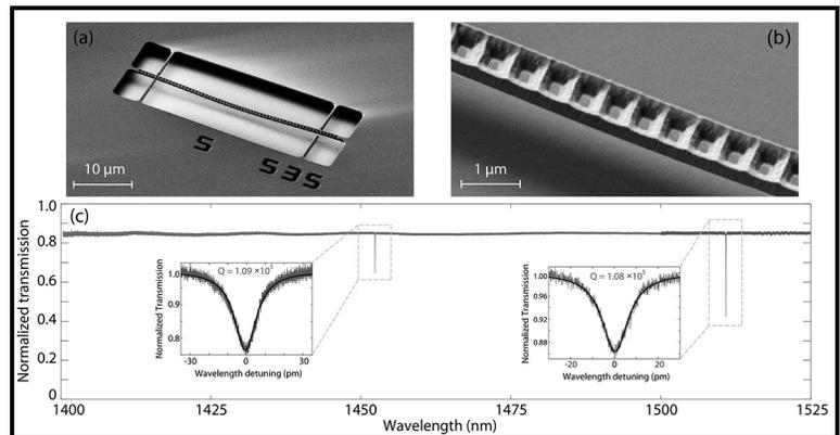
Figure 1: (a) (b) SEM images of a  $\text{LiNbO}_3$  photonic crystal nanobeam. (c) Normalized transmission spectrum of the photonic crystal cavity, measured by two tunable lasers operating at different wavelength ranges (indicated as black and grey curves). Insets show detailed transmission spectra of the fundamental TE ( $\text{TE}_0$ ) mode and second-order TE ( $\text{TE}_1$ ) mode, respectively.
