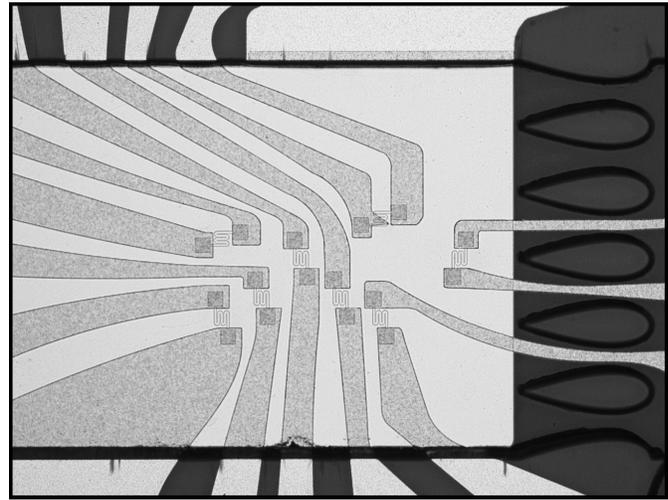
Figure 2: Microscopic image of hydrofoil array with pin fins, RTDs and electrical vias.
