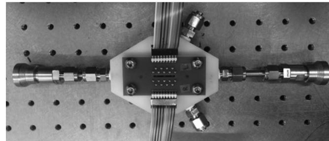
Figure 3: Package with external electrical connections.
