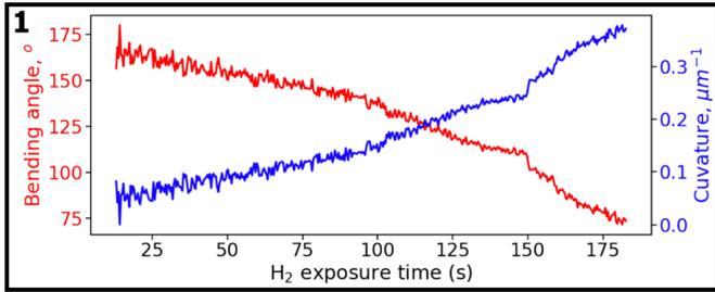
Figure 1: Hydrogen response for the Pd actuator hinge. Bending angle is defined as the angle between the two SiO<sub>2</sub> panels, and curvature is the change in the angle of deformation per unit length.
