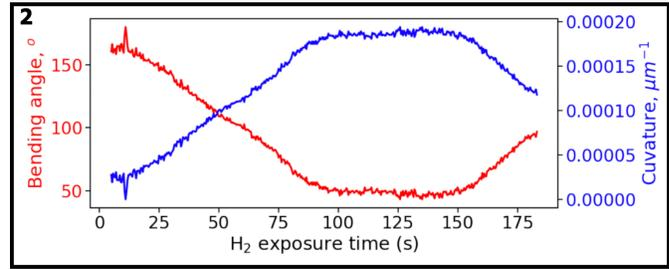
Figure 2: Hydrogen response for the palladium-gold actuator hinge.
