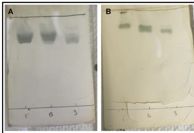
Figure 2: Early TLC plate tests. Figure 2A shows the initial TLC protocol. Figure 2B shows an improved protocol using a running solvent with chloroform/methanol/0.2% aqueous calcium chloride (60:40:10, v/v/v). All samples were suspended in methanol. For each plate, GM1 is spotted on the left, GM3 is spotted on the right, and there is a spot with both in the middle.
