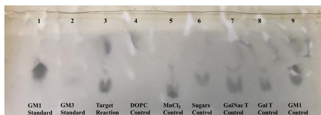
Figure 3: A TLC plate with the improved protocol. The top marks are likely other sugars or impurities. Columns 1 and 9 show GM1. Column 5 roughly indicates where GM3 is located. The remaining columns are GM2 intermediates.
