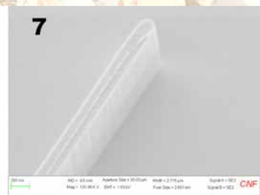
Figure 3: CH_2F_2 /He SiO_2 etch, 155 nm/min, Selectivity-4.4. Figure 4: CH_2F_2 /He SiO_2 etch, 155 nm/min, selectivity-5.8. Figure 5: C_4F_6 /He SiO_2 etch, 260 nm/min, selectivity-4.4. Figure 6: C_4F_6 /He SiO_2 etch, 260 nm/min, selectivity-4.4:1. Figure 7: TiO_2 / SiO_2 waveguide etched with C_4F_6 /He. Figure 8: TiO_2 / SiO_2 waveguide etched with C_4F_6 /He.
