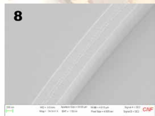
Figure 3: CH_2F_2 /He SiO_2 etch, 155 nm/min, Selectivity-4.4. Figure 4: CH_2F_2 /He SiO_2 etch, 155 nm/min, selectivity-5.8. Figure 5: C_4F_6 /He SiO_2 etch, 260 nm/min, selectivity-4.4. Figure 6: C_4F_6 /He SiO_2 etch, 260 nm/min, selectivity-4.4:1. Figure 7: TiO_2 / SiO_2 waveguide etched with C_4F_6 /He. Figure 8: TiO_2 / SiO_2 waveguide etched with C_4F_6 /He.
