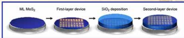
Figure 1, above: A schematic for fabrication of molybdenum disulfide/silicon dioxide stacking using alternating metal organic chemical vapor deposition growth, device fabrication with photolithography, and silicon dioxide deposition. Kibum Kang
