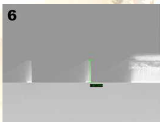
Figure 3: CH_2F_2 /He SiO_2 etch, 155 nm/min, Selectivity-4.4. Figure 4: CH_2F_2 /He SiO_2 etch, 155 nm/min, selectivity-5.8. Figure 5: C_4F_6 /He SiO_2 etch, 260 nm/min, selectivity-4.4. Figure 6: C_4F_6 /He SiO_2 etch, 260 nm/min, selectivity-4.4:1. Figure 7: TiO_2 / SiO_2 waveguide etched with C_4F_6 /He. Figure 8: TiO_2 / SiO_2 waveguide etched with C_4F_6 /He.
