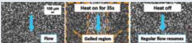
Figure 2: Dynamic channel creation and reconfiguration. A narrow straight channel created within a larger microfluidic chamber by selective heating along the sides. The original flow field was obtained on turning the heat off.
