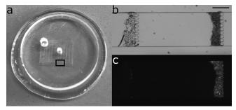
Figure 1: Microfluidic chip. a) Completed microfluidic chip with inlet at center and outlet on the left. Box depicts pillar/bead zone. b) Microscope image of channels, pillars, and different sized bead zones c) Microscope image of fluorescence on beads after flowing of AlexaFluor488 through chip.
