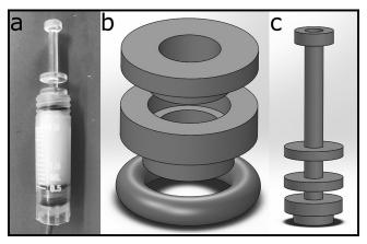
Figure 3: Saliva filtration setup. a.) Image of complete filtration setup. b.) Custom filter holder with two pieces that hold a circular filter between them and an O-ring beneath. c.) Plunger to compress saliva swab and push saliva through filter.
