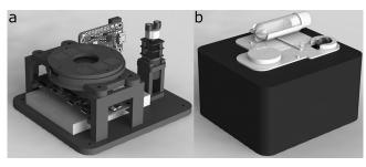
Figure 2: Rendering of 3D-printed imaging and pumping device. a) Interior assembly including Raspberry Pi Zero W, optical components, geared motor, custom peristaltic pump head, lithium-ion battery, and Powerboost 1000C. b) Exterior of device with disposable cassette attached via snap fit.
