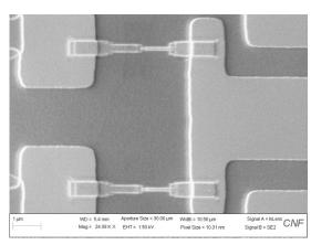
*Figure 1: Scanning electron micrograph of Al-AlO<sub>x</sub>-Al Josephson junctions in protected qubit design.*
