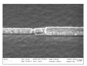
Figure 2: Scanning electron micrograph closeup image of Al-AlO<sub>x</sub>-Al Josephson junction on protected qubit element.
