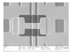
Figure 3: Scanning electron micrograph of Nb ground connection over SiO<sub>2</sub> spacer on protected qubit element.
